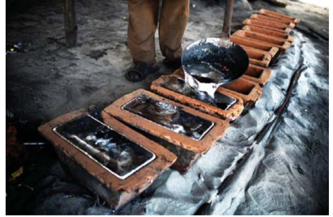
Worker pours liquid aluminum into casts at a recycling factory.
