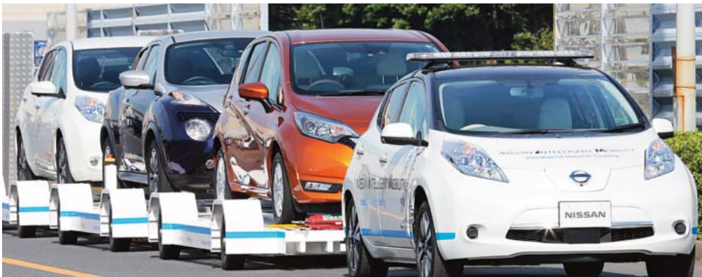
YOKOHAMA: Nissan Motor Co's "Leaf", with no one inside, pulls a trailer with three other Leafs on it, during a demonstration of the automaker's Intelligent Vehicle Towing system at Nissan Oppama plant. — AP
