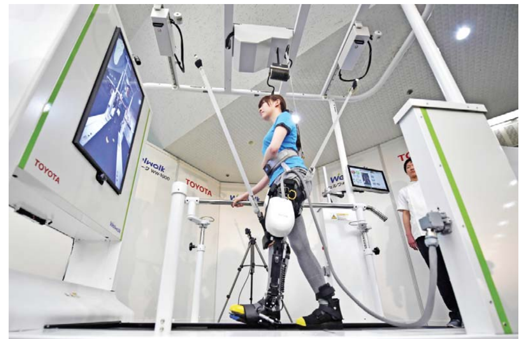
TOKYO: A model demonstrates how the rehabilitation-assist robot Welwalk WW-1000, developed by Japan's Toyota Motor Corporation, helps to assist in flexing and extending the knee while walking on a treadmill during a press preview in Tokyo yesterday. — AFP
