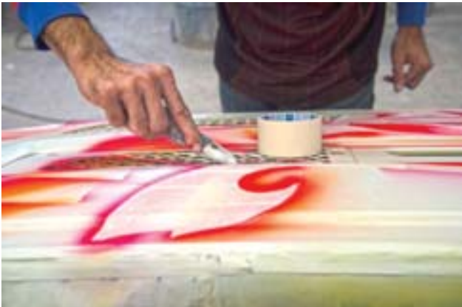
This photograph shows a painter cutting away a masking tape for a stencil design on a truck panel.
