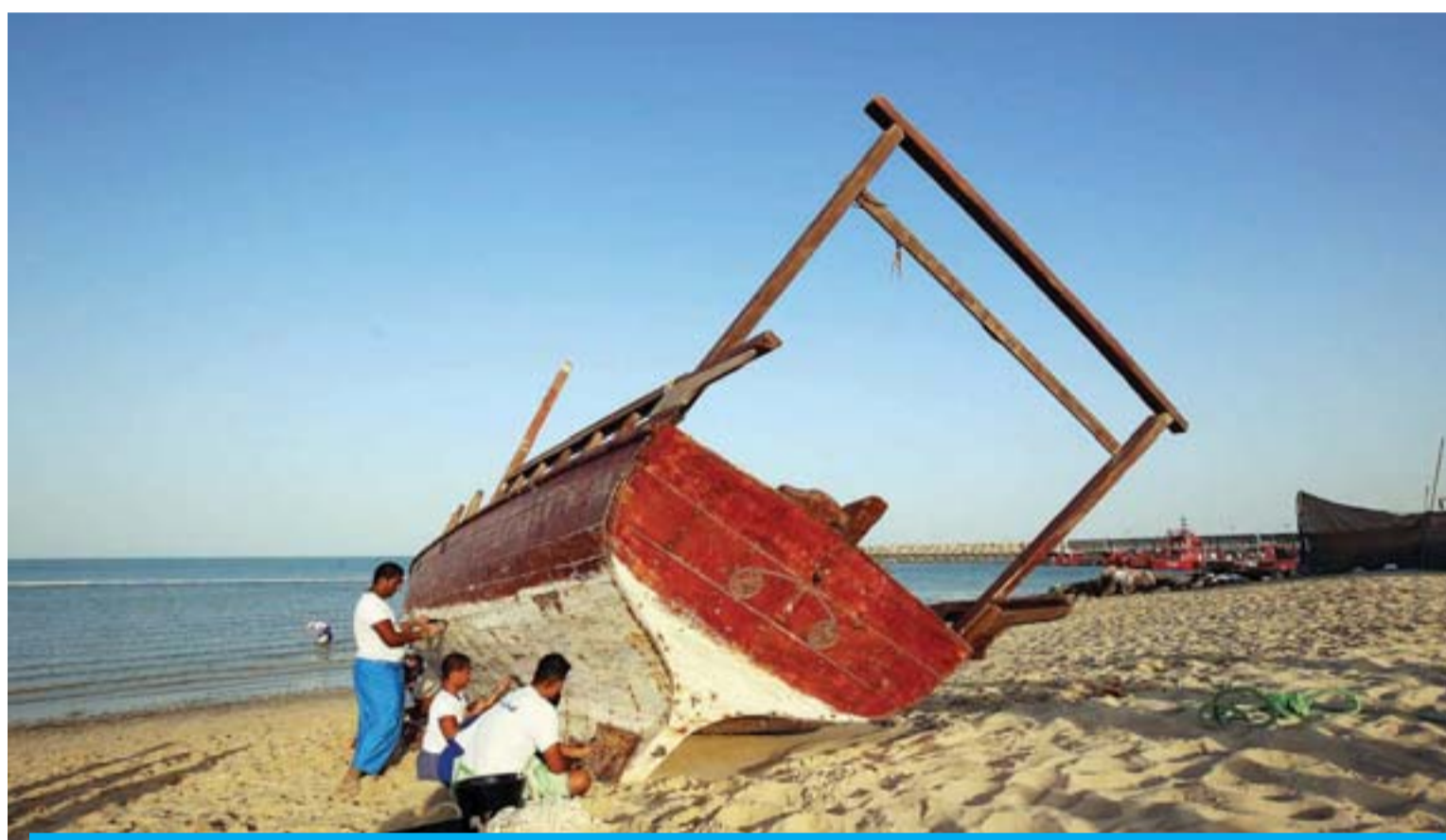
KUWAIT: Sailors apply a mixture of white cement and animal grease (habab and shouna) to the body of a dhow yesterday as part of preparations for the pearl diving festival. Pearl-diving trips are held annually under the patronage of HH the Amir in order to keep alive traditions that accompanied the once important national trade of pearl diving, prior to the discovery of oil. — Photo by Yasser Al-Zayyat (See Page 4)
