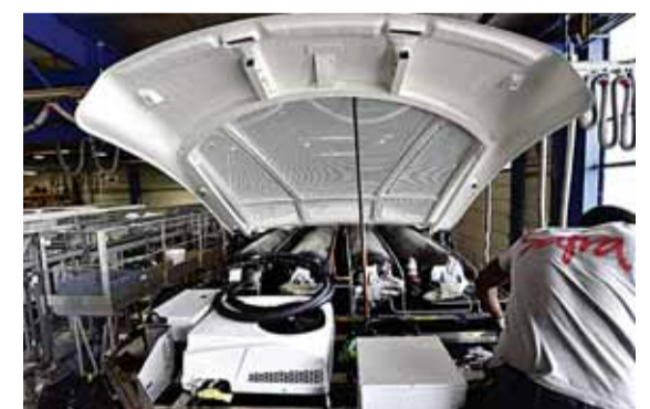
A technician works on the hydrogen tank of an under construction hydrogen bus, at the plant of the Albi's Automobile Company for Repair and Manufacturing (Societe Albigeoise Fabrication Reparation Automobile - SAFRA), in Albi, southwestern France.—AFP
