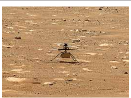
NASA's Ingenuity helicopter unlocks its rotor blades, allowing them to spin freely, on April 7, 2021, the 47th Martian day, or sol, of the mission, captured by the Mastcam-Z imager on NASA's Perseverance Mars rover on the following sol, April 8, 2021. —AFP
