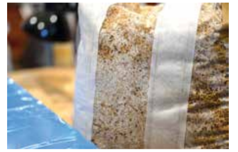
A bag of mycelium and cornhusks used to mold a guitar body sits in French luthier Rachel Rosenkrantz's studio.
